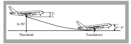
Typically, the pitch attitude increases slightly during the actual landing, but avoid over-rotating. Do not increase the pitch attitude after touchdown; this could lead to a tail strike.
