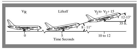
Retract the landing gear after a positive rate of climb is indicated on the altimeter. Retract flaps in accordance with the technique described in this chapter.
